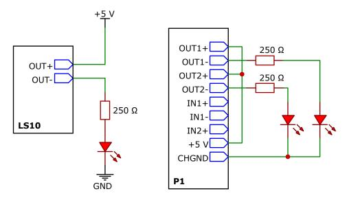
When the GPO is **closed**, the LED is **turned on**.
