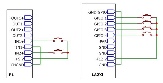
When the push button is closed, the GPI logic state is HIGH.
