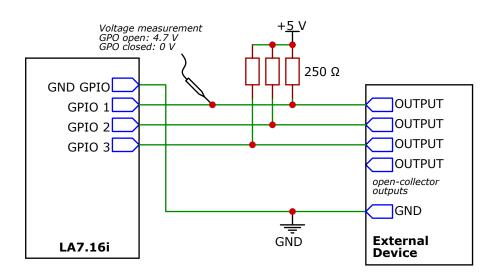
The open-collector output is either floating or connected to ground. Pull-up resistors are used to force the **HIGH** logic state when the output is open.
