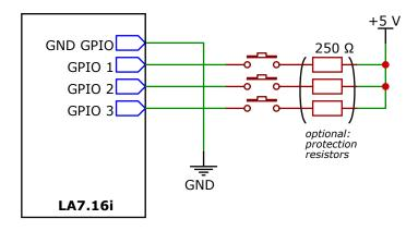
When the push button is closed, the GPI logic state is HIGH.
