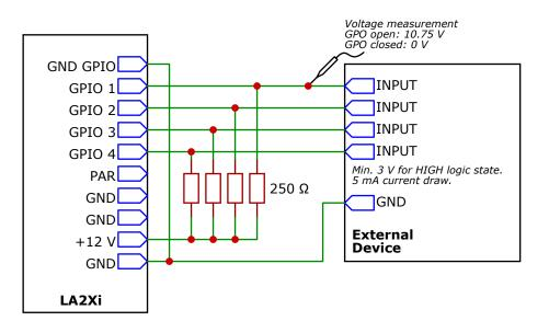
When the GPO is **closed**, the GPI of the external device is set to **LOW** logic state.
