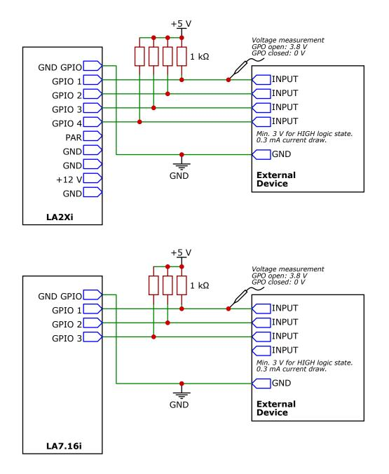
When the GPO is **closed**, the GPI of the external device is set to **LOW** logic state. When the GPO is **open**, the GPI of the external device is set to **HIGH** logic state.
